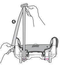
4. Slide the vehicle shoulder belt onto the clip as shown **3** and pull free end of strap down **3** to tighten clip against the child's shoulder.
